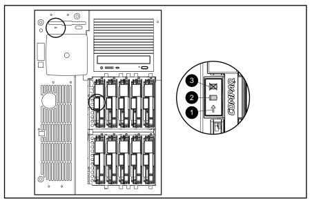
Figure 4-13. Hot-plug hard drive LED indicators
